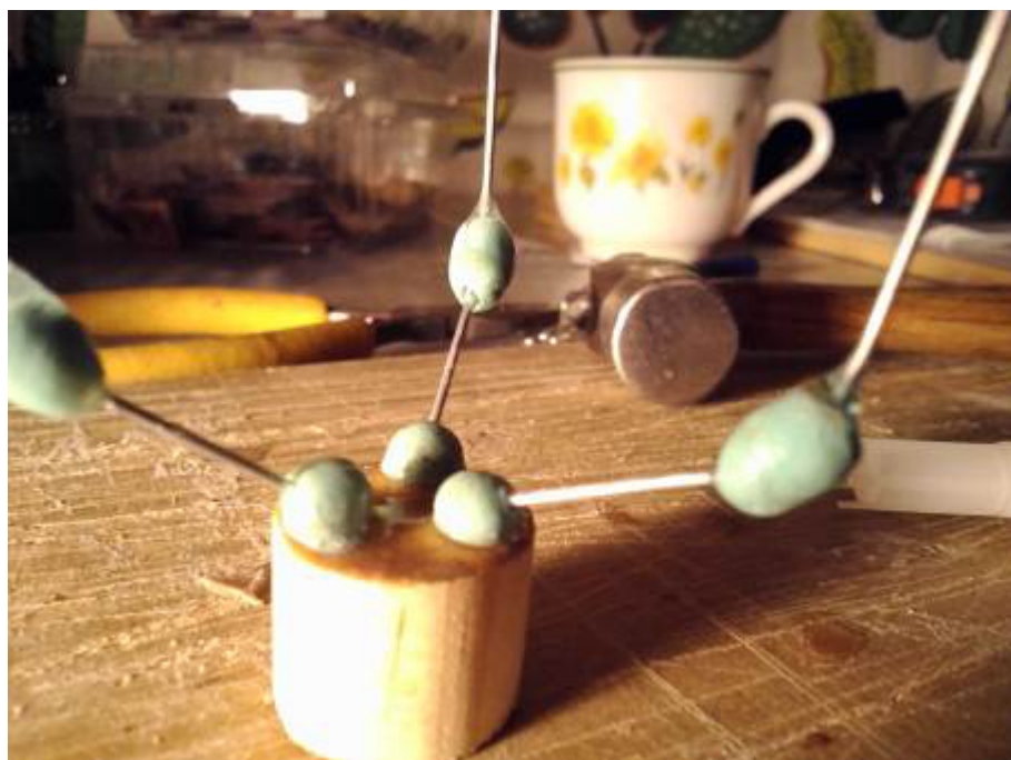
The Blu Tack joints close up. I even made the super-glue generate a smooth transition between joints and the legs.
